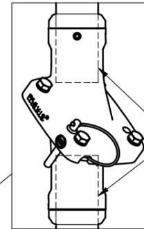
PIPE SECTIONS ARE INSERTED INTO Maxis™ JOINT
