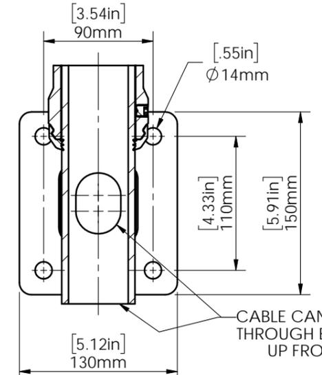
CABLE CAN BE ROUTED THROUGH BRACKET OR UP FROM BASE.
